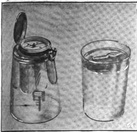
This Photo Shows the Jewelled Bearing Magnet Compass and One of the Earliest Forms of a Compass, Formed of a Piece of Magnetized Steel Resting on the Surface of a Glass of Water. A Steel Needle Was Magnetized by a Lodestone and Dropt Gently into the Water in Early Times, but in This Case a Steel Writing Pen Was Employed. Try the Needle Trick Yourself. We Found It Most Interesting. It Points to the North.
