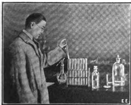
Nesslerizing Water in the Ammonia Determination. Nessler's Reagent Is Being Introduced With a Pipette.
