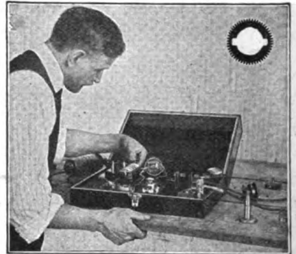
This Instrument Quickly Locates Defects Or Trouble in the Various Parts of Automobile Magnetos. By Means of This Instrument, You Can Quickly and Accurately Locate Trouble in the Condenser, Collector, or Armature.
